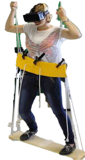
Fig. 1. Intermediate prototype from the iterative design process for a range of suspended setups for locomotion in VR.
