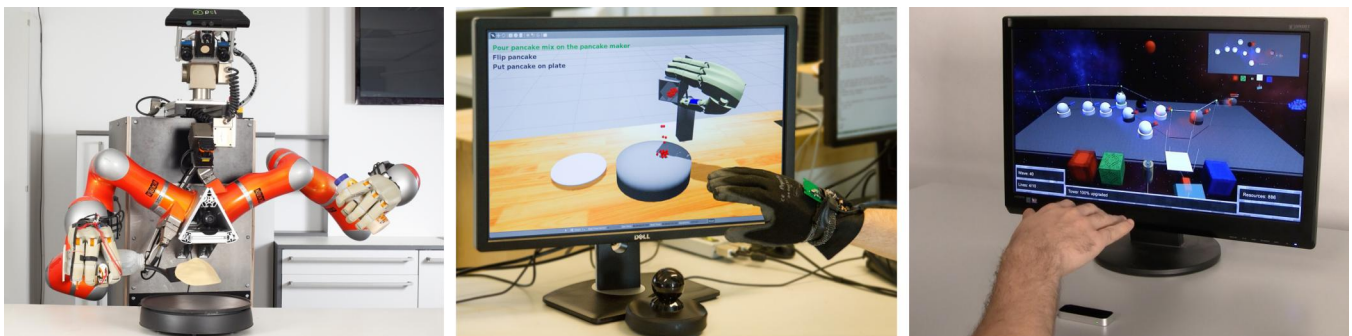
Figure 1: Many robot manipulation tasks (left) are learnt best by observing humans. Human motion can be demonstrated using virtual environments (center). Data acquisition with motion-based games makes demonstrating a fun activity (right).
